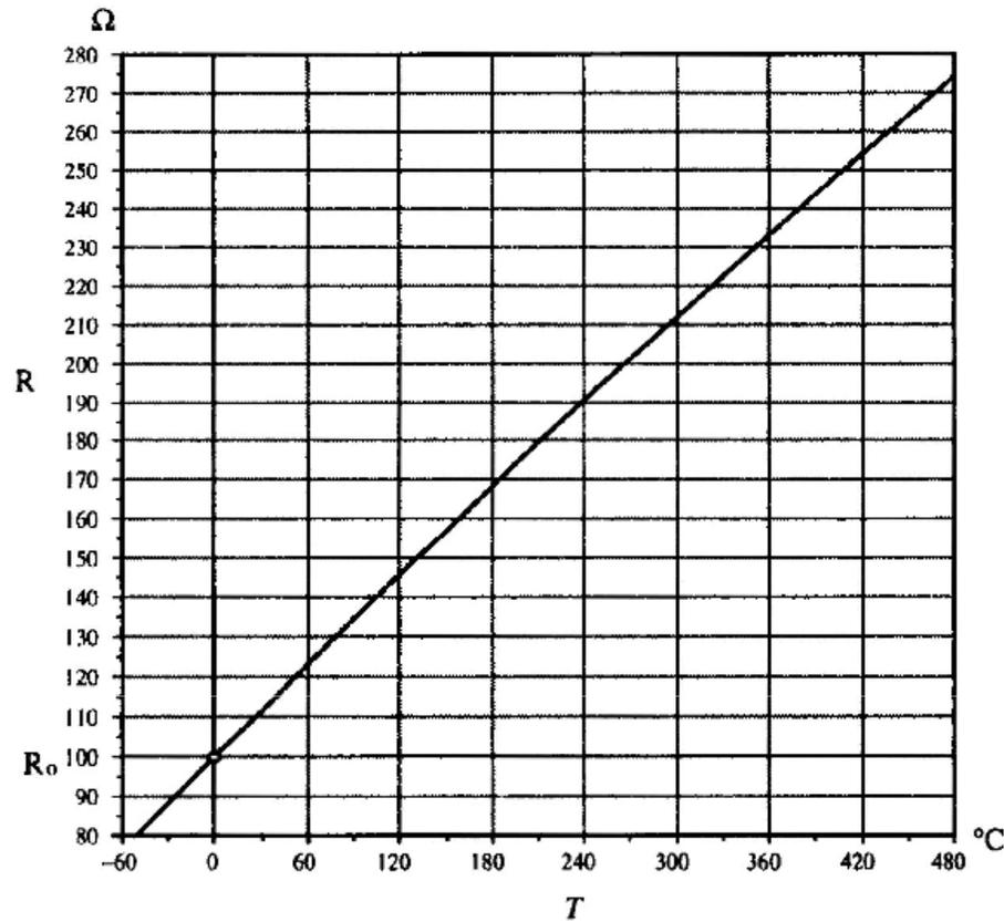
FIGURE 3.18. Resistance of platinum as function of temperature.
