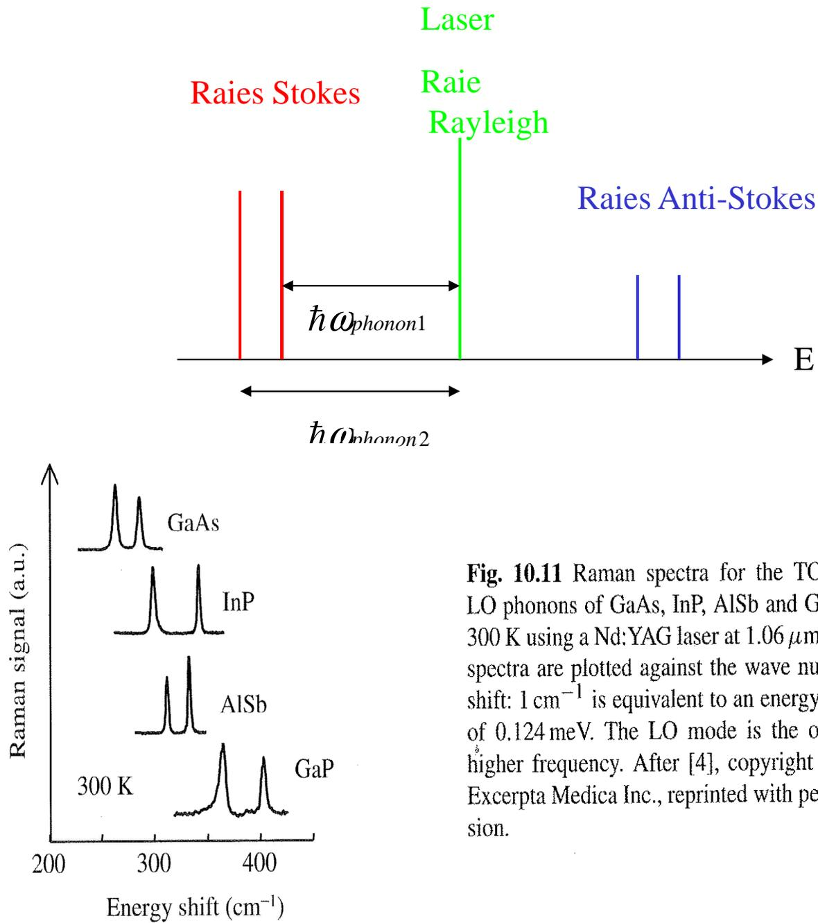
**Fig. 10.11** Raman spectra for the TO and LO phonons of GaAs, InP, AlSb and GaP at 300 K using a Nd:YAG laser at  $1.06\ \mu m$ . The spectra are plotted against the wave number shift:  $1\ cm^{-1}$  is equivalent to an energy shift of  $0.124\ meV$ . The LO mode is the one at higher frequency. After [4], copyright 1972 Excerpta Medica Inc., reprinted with permission.
