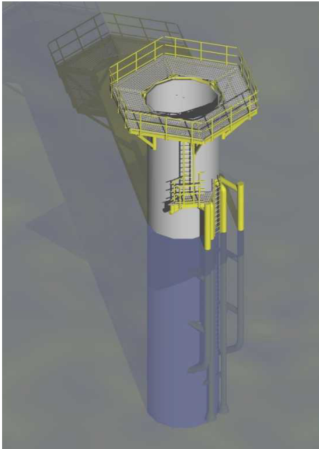
Figure 8-14. Monopile Foundation, from LIC Engineering (1997)
