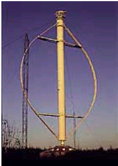
Figure 1-2. Eole C, a 4200 kW vertical axis Darrieus wind turbine with 100 m rotor diameter at Cap Chat, Québec, Canada. The machine, which is the world's largest wind turbine, is no longer operational. From www.windpower.org (2000), © Danish Wind Turbine Manufacturers Association.
