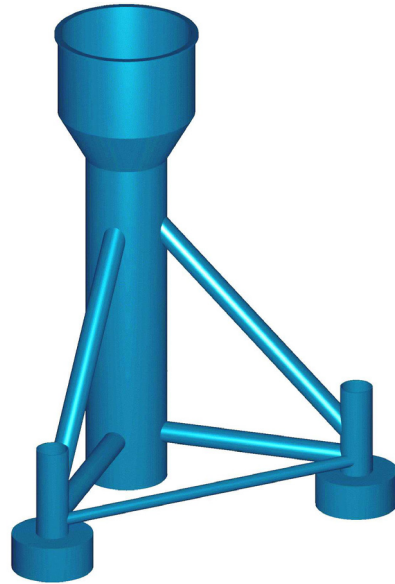
Figure 8-17. Tripod with suction buckets, from Rambøll (1998).
