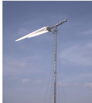
Figure 1-10. A conception of a flexible wind turbine. During stand-still, the blades deflect as a rush in the wind.
