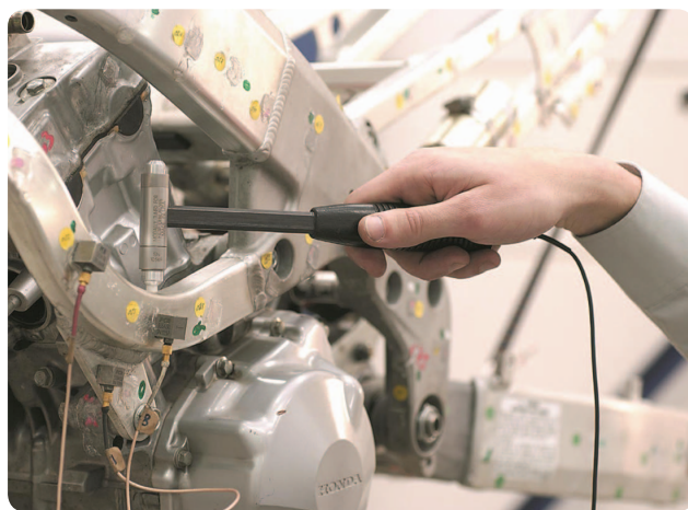
FIGURE 16 Hammer excitation in a mechanical vibration analysis in the vibration labs of Siemens Industry Software Leuven, Belgium. A force transducer is placed in the tip of the hammer that allows the impact force to be measured. Accelerometers are mounted on the mechanical structure to measure the response of the system. (Used with permission from Siemens.)
