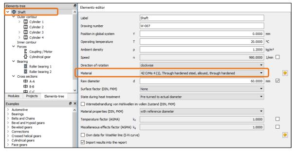
Figure 19. Shaft material
