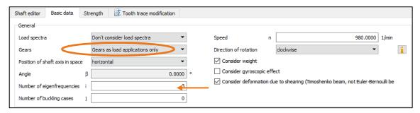
Figure 11. Inputting the number of eigenfrequencies
