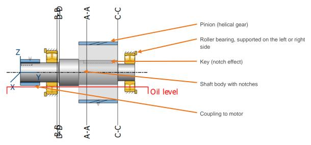
Figure 3. Analyzed pinion shaft
