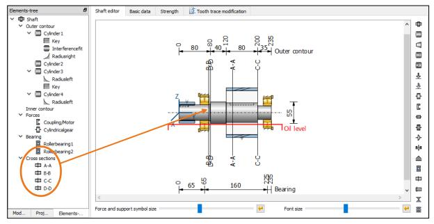
Figure 23. Cross sections to be analyzed
