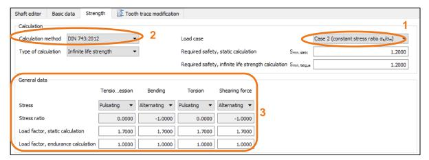
Figure 15. Buttons involved in strength calculation
