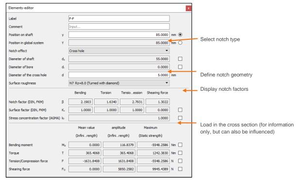
Figure 27. Definition of notch in cross section F-F
