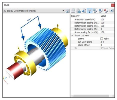
Figure 14. 3D display of deformation (bending)
