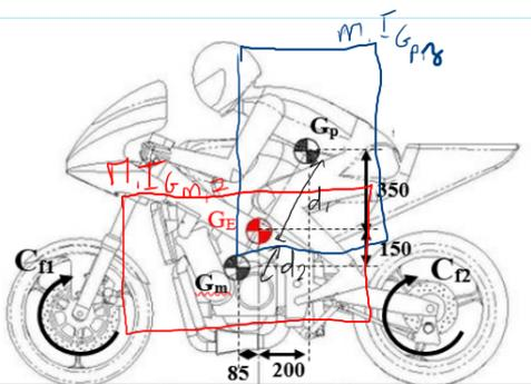
$$I_{G_{E,z}} = I_{G_{p,z}} + m \cdot d_1^2 + I_{G_{m,z}} + m \cdot d_2^2$$
