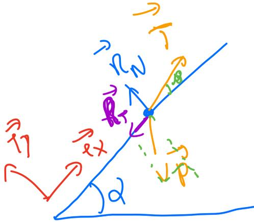
$$\begin{aligned} \vec{R} &= \begin{pmatrix} -R_T \\ R_N \end{pmatrix} \\ \vec{T} &= \begin{pmatrix} T \cos \beta \\ T \sin \beta \end{pmatrix} \\ \vec{P} &= \begin{pmatrix} -mg \sin \alpha \\ -mg \cos \alpha \end{pmatrix} \end{aligned}$$
