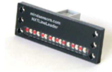
Figure 4: The LineLeader sensor
