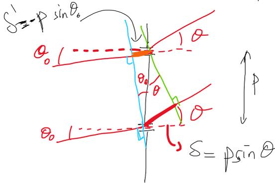
$$\left. \begin{aligned} \delta &= p \sin \theta_0 \\ \delta &= p \sin \theta \end{aligned} \right\} \Rightarrow \begin{aligned} \delta_T &= n_2 - n_1 \\ &= \delta + \delta' \\ &= p [\sin \theta - \sin \theta_0] \end{aligned}$$
