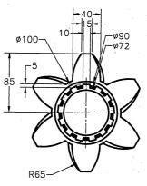
The plane for drawing the second section is at an offset of 45mm from the first sketch. Plane for the third sketch is at an offset of 50mm from the second sketch
