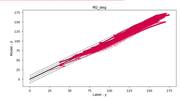
This graph shows the temperature predicted by the tnn as a function of the targe temperature. the closer the data (in red) are to the bisector, the more successful the prediction.
