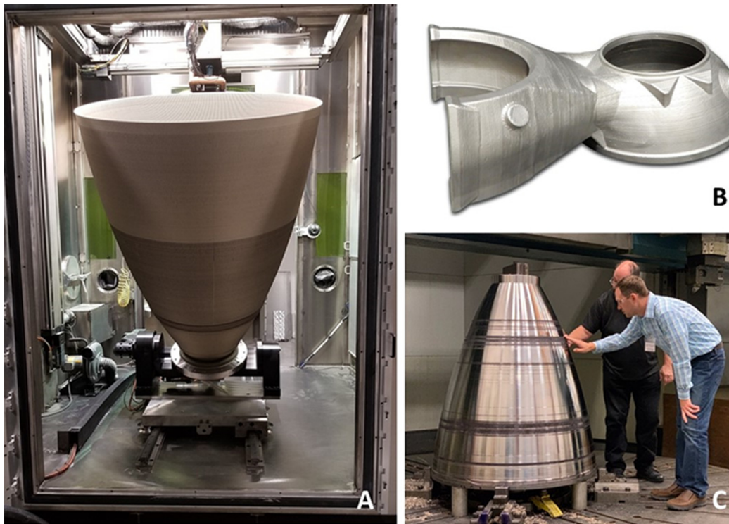
Fig. 21. Examples of Large Scale DED at NASA. A) LP-DED integral channel nozzle 60" (1.52 m) diameter and 70" (1.78 m) height with NASA HR-1 alloy deposited in 90 days, B) Powerhead half shell using Inconel 718, and C) LP-DED JBK-75 Nozzle (no channels) that is ½ scale RS-25. (Courtesy: NASA)[212].
