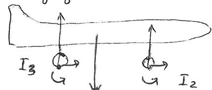
$$\sum \vec{M}_{I_2 ext, \varepsilon} = \vec{\delta}_{I_2} (\varepsilon / R_g) \rightarrow \vec{\delta}_{I_2, 1/R_g} = -M \ddot{x} \cdot h$$
