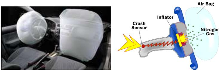
Figure n° 1 – Airbag principle
