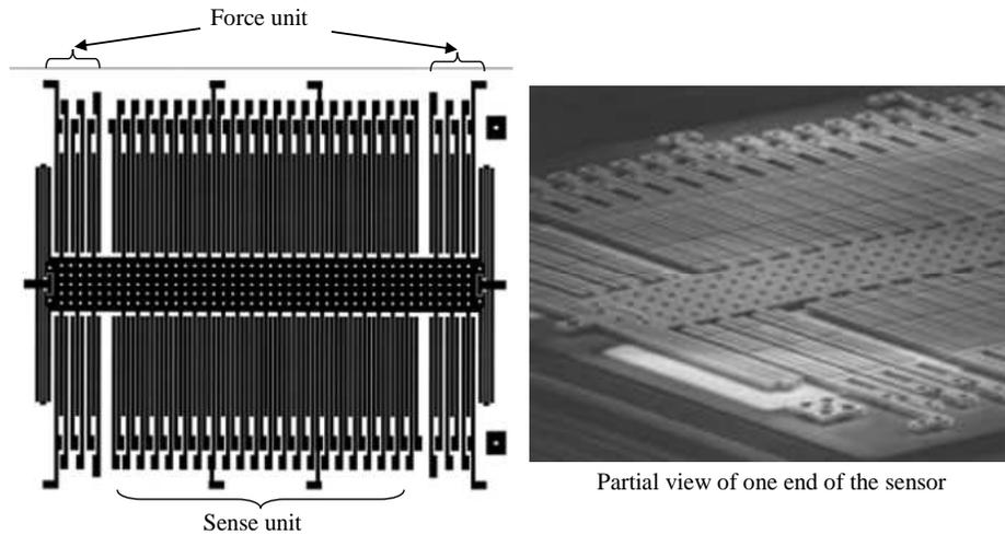
Figure n° 3 – Silhouette plots of ADXL150 sensor. Axis of motion is horizontal
