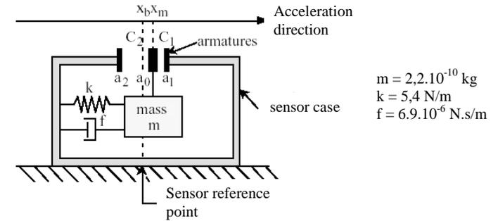
Figure 5 - Mass-Spring system used for measuring acceleration
