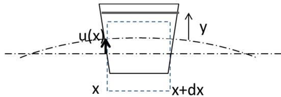
Figure 7 – Flexural deformation
