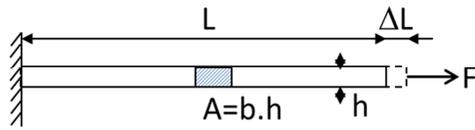
Figure 6 – Traction/compression beam
