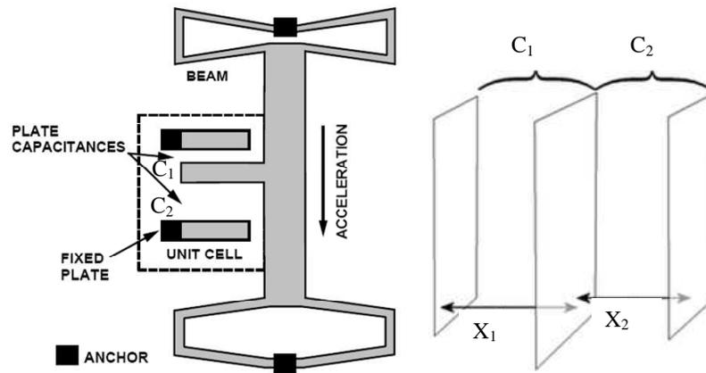
Figure n° 4 – The dual Capacitor system used to measure displacement in the Analog Devices ADXL50 accelerometer
