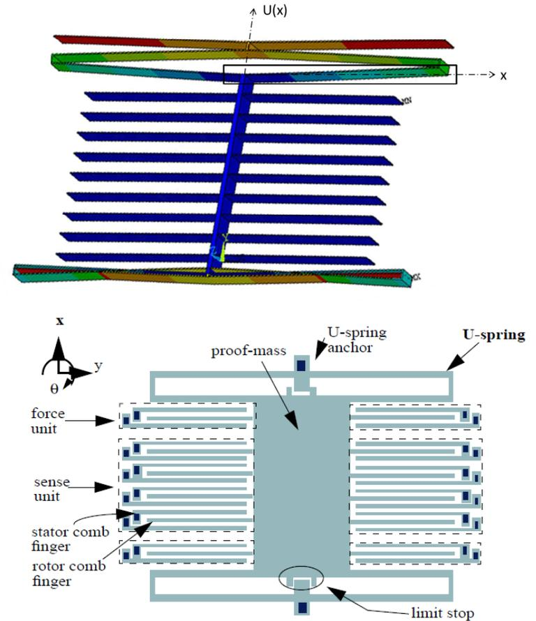
Figure 8 – U-spring deformation
