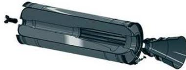
Figure 2 –The first stage of the Vega launcher (motor and the nozzle) – P80
