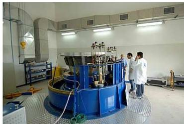
Figure 3 – Validation test of the P80 thrust vector control system
