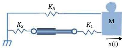
Figure 2. Equivalent translational model of the nozzle
