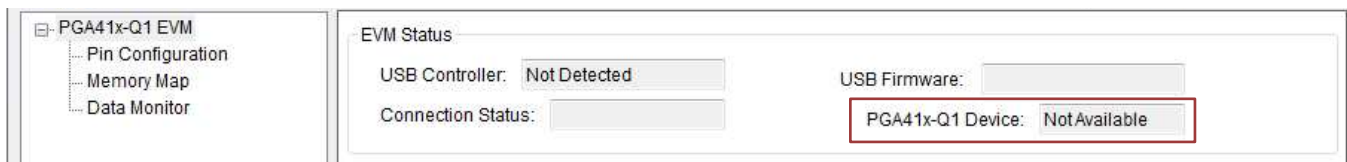
Figure 4. PGA411-Q1 Device Startup Failed
